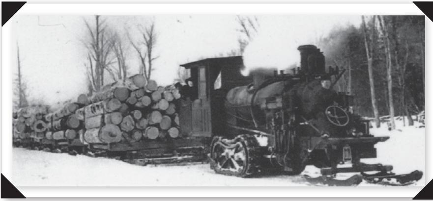
An early Phoenix Log Hauler, steam powered, no headlight. Light was provided by a kerosene lantern at the drivers feet.
